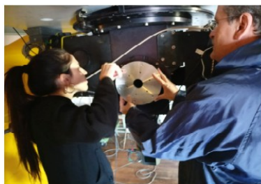
Figure 4: Mounting the PAT in the East port
